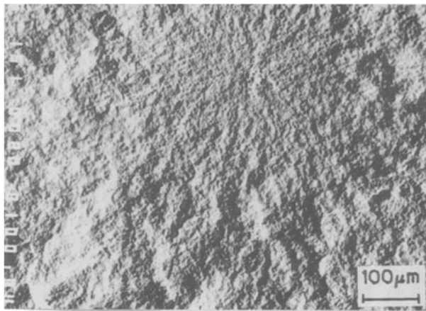
Figure 10 Scanning electron micrograph of a specimen oxidized at 1300°C for 100 h in a wet atmosphere of 40 vol% H 2 O. Failure occurring at a coarse grain in the subsurface.
